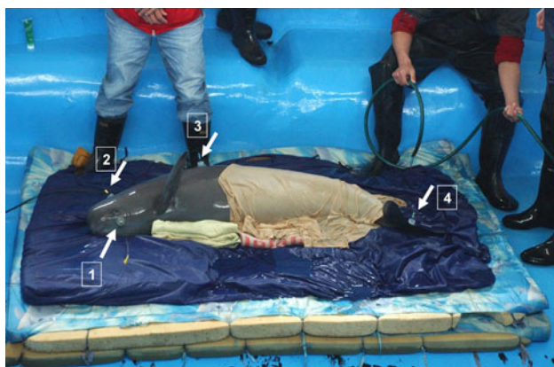
Fig. 1 Experimental setup. During the hearing tests, the respective porpoise was situated out of the water on several foam mats and kept moist using wet towels and continuous watering via a hose. Sound was presented using a suction cup jawphone (1). Responses were recorded using a three electrode configuration with the non-inverting electrode (2) just behind the blowhole, the ground on the animals back (3) and the inverting electrode on the fluke (4)
