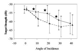
Figure 1. Target strength in dB re:  $1\mu Pa$  of barium sulphate and nylon nets; solid line: barium sulphate net; dashed line: nylon net. Error bars represent standard deviations of the mean for TS measurements. Statistically significant results are marked with a star.
