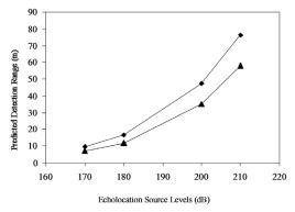
**Figure 2.** Predicted maximum detection range of a barium sulphate net at normal incidence at increasing source levels (dB re:  $1\mu$ Pa) by *Tursiops truncatus*; diamonds: 27dB of noise; triangles: 33 dB of noise
