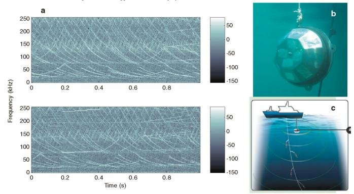
**Fig. 2.** (*a*) Sample spectrograms of the various acoustic signals produced by the acoustic deterrent. (*b*) The *Long-line Saver* hung in sea water for calibration. (*c*) A diagram for the suggested use and deployment of the device.
