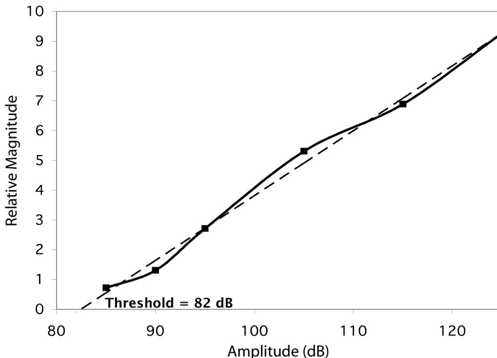
**Figure 4.** An example of threshold evaluation at 16 kHz for the FFT data of Figure 3; the solid line and points are actual measured data points, and the checked line is a linear regression line, which, when the zero point is calculated, assigns the threshold for this frequency at 82 dB.
