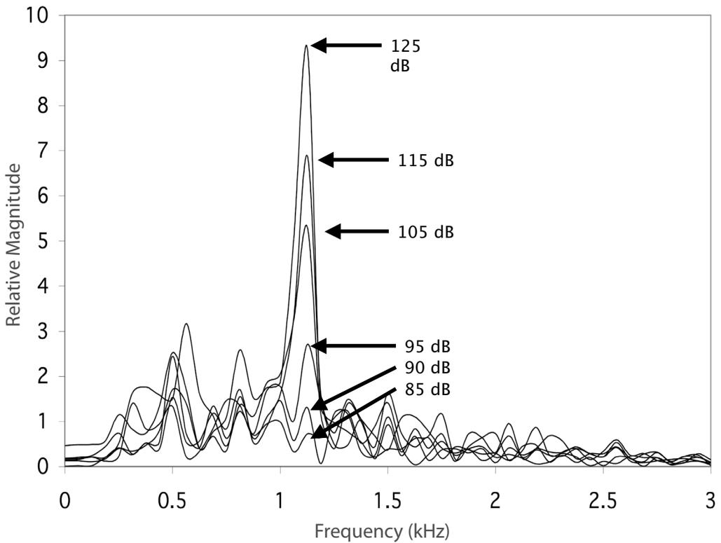
**Figure 3.** Fast Fourier transform (FFT) of the waveforms from Figure 2; the FFT response magnitudes are a relative measure of the acquired waveforms. Note the decreasing amplitude of the FFT with decreasing stimulus amplitude.
