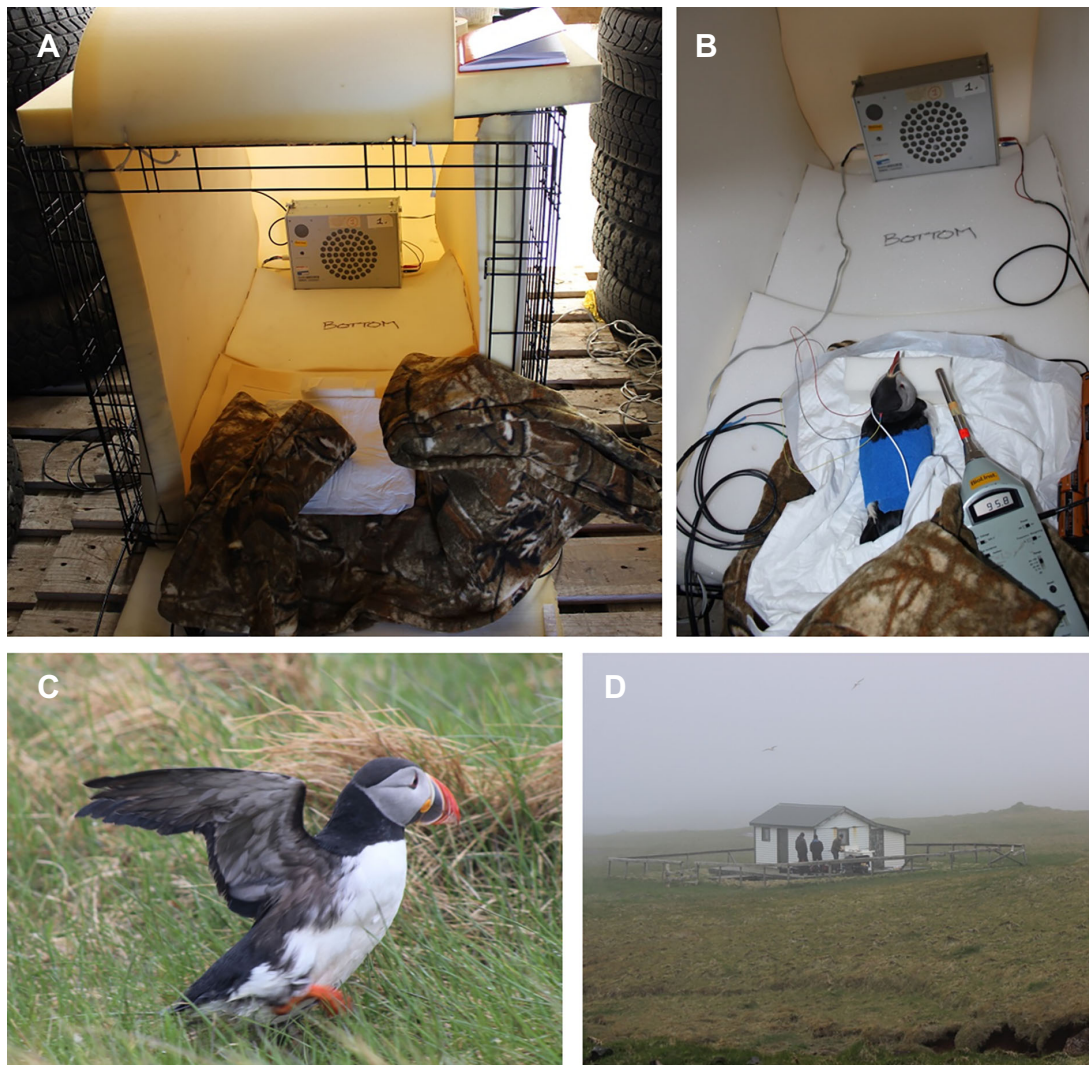
Fig. 1. Experimental setup and animal tested. (A) The semi-anechoic chamber lined with acoustically insulating foam. The speaker is at the far end, with heated blanket and bed-pad near the door. (B) The puffin during the AEP hearing test resting on a bed-pad and heated blanket. Electrodes are in place with the active electrode near the left ear. The sound level meter is to the right of the bird's head. (C) The puffin after release. (D) The location of the murre hearing test, Langanes peninsula, Iceland. The cabin offered a windbreak and is within 200 m of the rookery cliffs.
