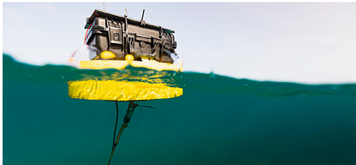
An acoustic electronics package floats on surface buoy above the reef. (Photo by Dan Mele, © Woods Hole Oceanographic Institution)
