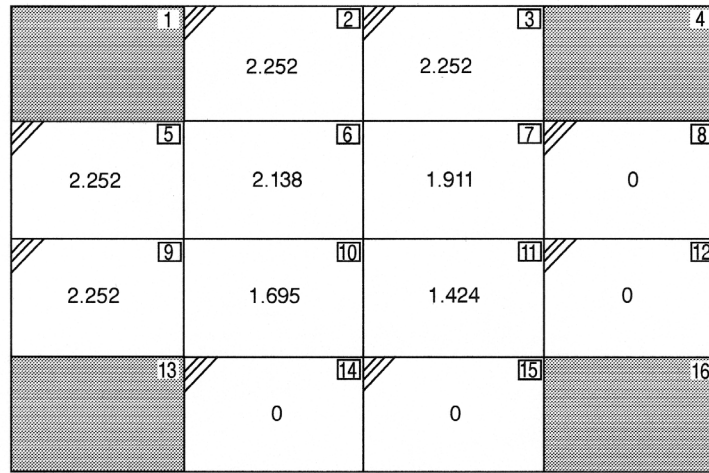
FIGURE 14. Terminal time concentrations (corresponding to the time histories in Figure 8), representing the terminal constraint (within error bars) of the control problem for transient tracers.
