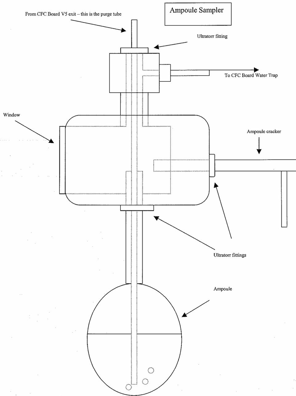
Figure 12. CFC Ampoule Sampler Schematic 1.
