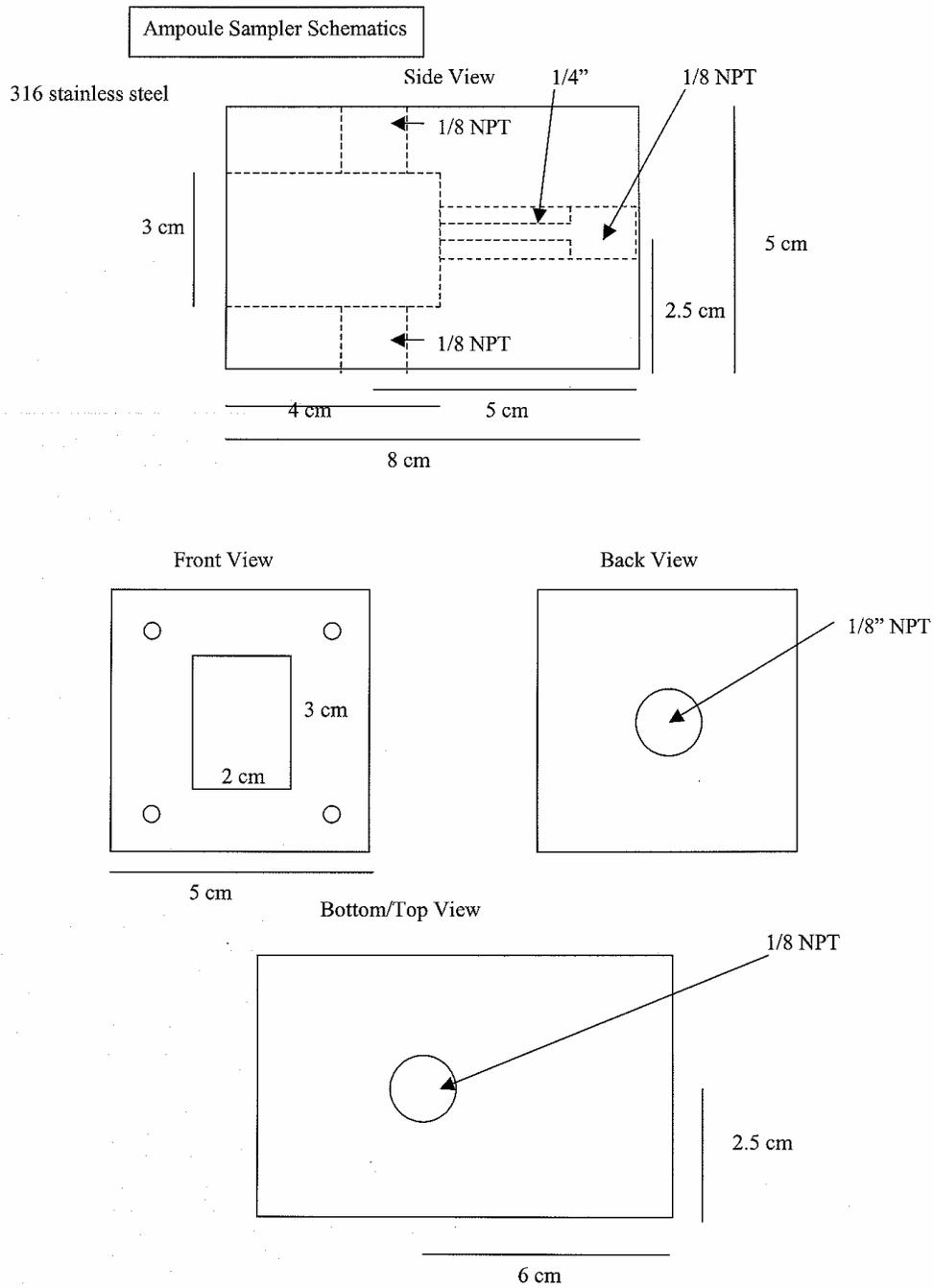
**Figure 13. CFC Ampoule Sampler Schematic 2.**
