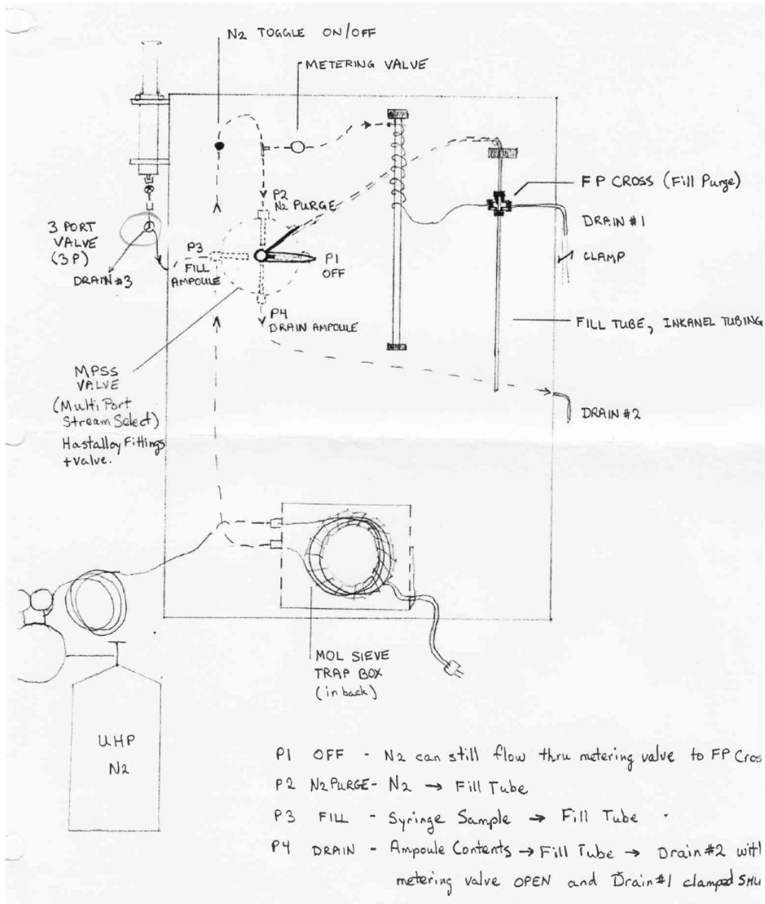
Figure 11. CFC Ampouler Diagram.
