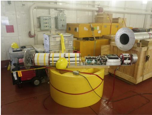
Figure 1: The instrumentation for the O-buoy. Starting from the left of the picture the tray holds: 3 Li battery packs for power during winter months when the solar array does not work, CO<sub>2</sub> tanks used as standards for the CO<sub>2</sub> sensor, the ozone detector and supervisory computer which controls buoy operations, the CO<sub>2</sub> sensor, and finally the spectrometer for the differential optical absorption spectroscopy done by the buoy to detect BrO
