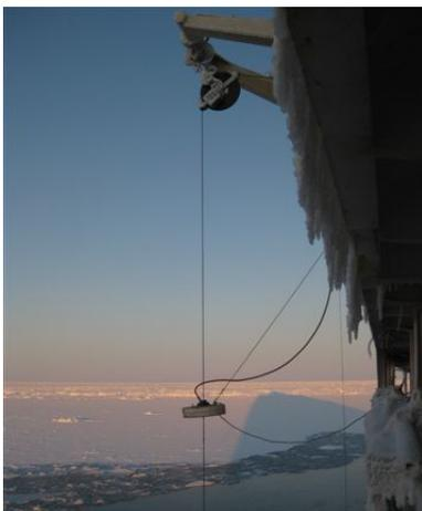
**Figure 8. The 'de-icer' attached to the CTD wire.**
