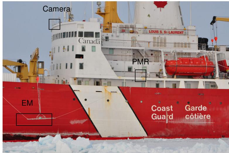
**Figure 1.** Pictures of EM , PMR and forward-looking camera.
