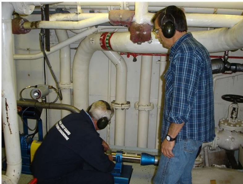
**Figure 2.** Pump for seawater loop at intake in engine room.
