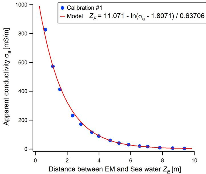
**Figure 3.** Result of EM calibration over open water.
