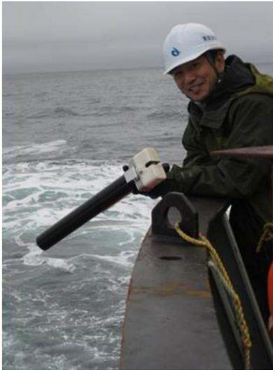
**Figure 1:** Kohei Mizobata deploying XCTD probe from the ship's stern
