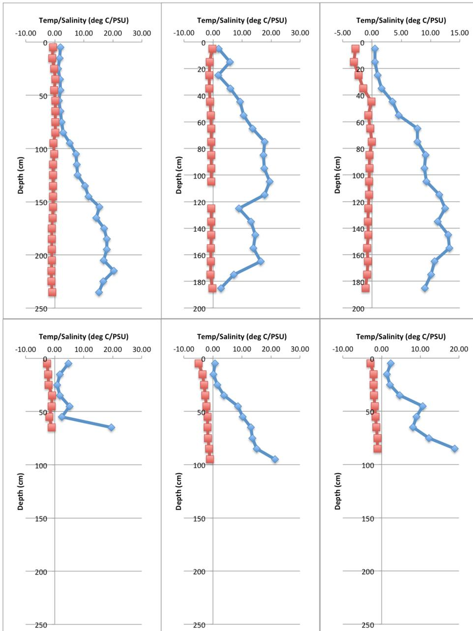
**Figure 6: Temperature (red)/Salinity (blue) profiles for the sampled cores. Top row: IBO 1, Cores 1-3 (left to right), bottom row: IBO 2, Cores 1-3 (left to right)**
