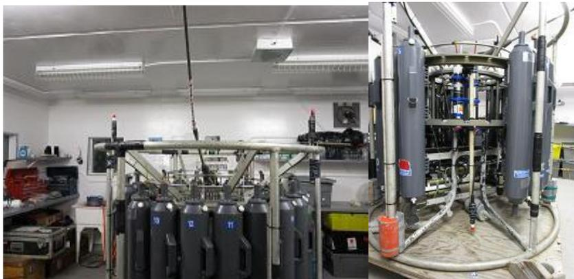
**Figure 2** Chipods mounted on the rosette.
