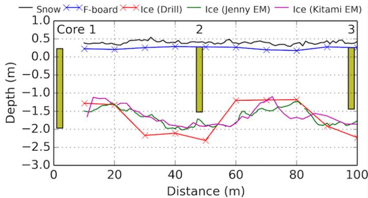
**Figure 4: Example transect from Ice Station 1. Black line is snow depth (every 1m), red crosses are the drilled ice thickness, blue crosses are the freeboard depth and the green and blue lines are the thicknesses obtained from two different EM sensors pulled along the transect line. The data was converted into depth using the snow and freeboard data. Raw data is available on the ScienceNet server.**
