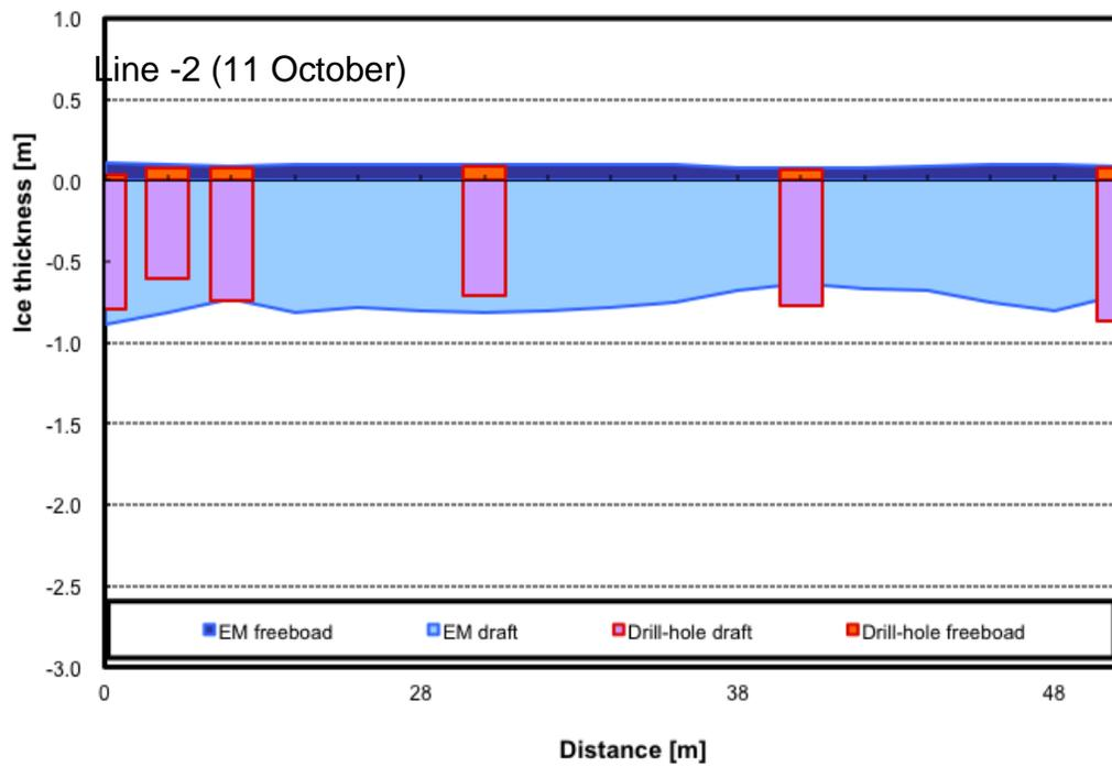
Figure 5. Comparison of EM31SH with drill-hole thickness measurements at Ice Station #1 on 6<sup>th</sup> of October 2014 and #2 on 11<sup>th</sup> of October 2014.
