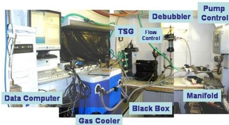
**Figure 9. Seawater loop system**
