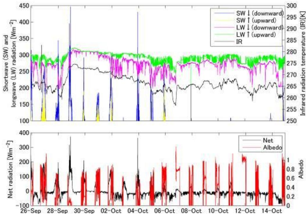
We found out the unusual albedo data (over 1) in 26-27 September and 7-14 October. It is necessary to calibrate because these are affected the shortwave radiation shutdown and the influence of longwave radiation by ship.
