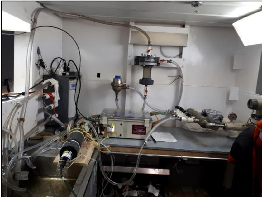
**Figure 19.** Seawater loop system in 2020, includes the new FDOM sensor – similar for 2021. The seawater loop provides uncontaminated seawater from 9m depth to the science lab for underway measurements
