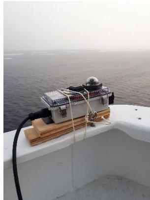
Self-contained camera system with solar panel mounted above the bridge on forward, port corner.
