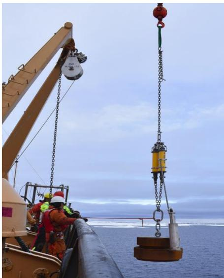
**Figure 1. Recovery of top floatation package, MMP deployment, and anchor, acoustic release, and BPR deployment.**
