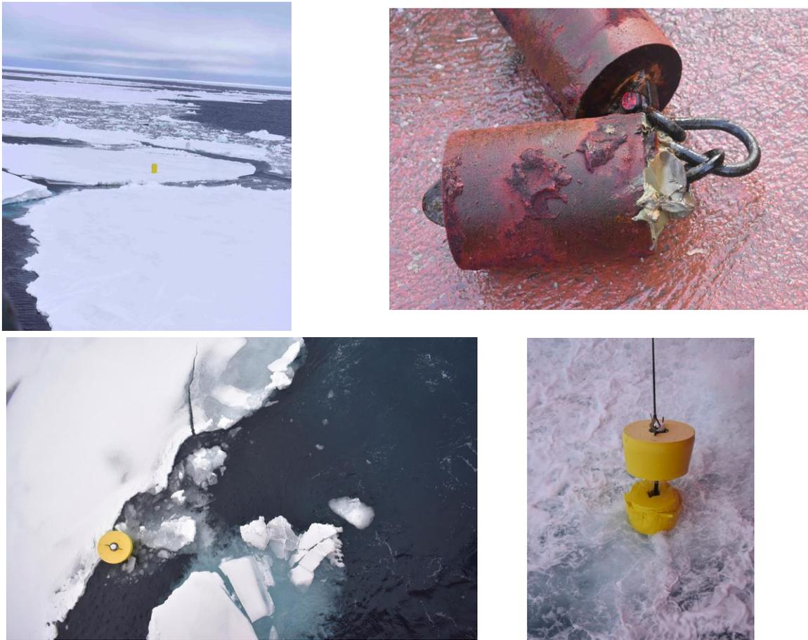
**Figure 3. ITP 119 recovery location (top left) and its muddy anchors (top right), ITP 112 recovery location (bottom left), and its severed top floatation (bottom right).**
