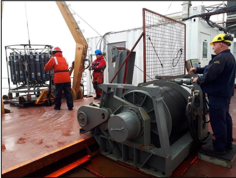
**Figure 9. Rosette operation on deck with Hawboldt winch and Brooks Ocean Instrumented Sheave display box mounted on the right.**
