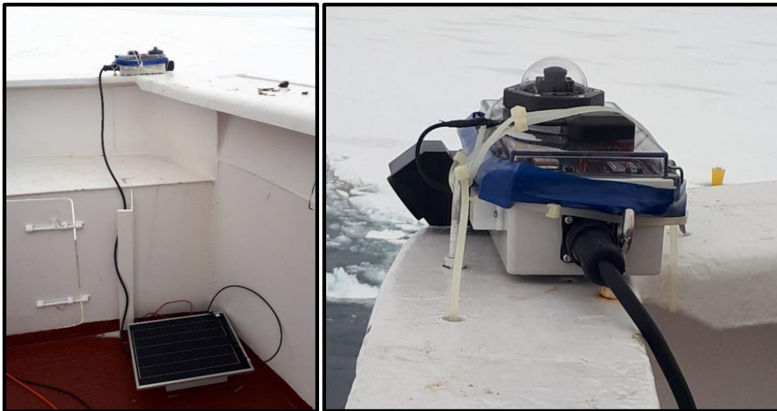
Figure 34. Self-contained camera system with solar panel mounted above the bridge on forward, port corner. Photos from 2022 but similar to 2023 but without the solar panel.
