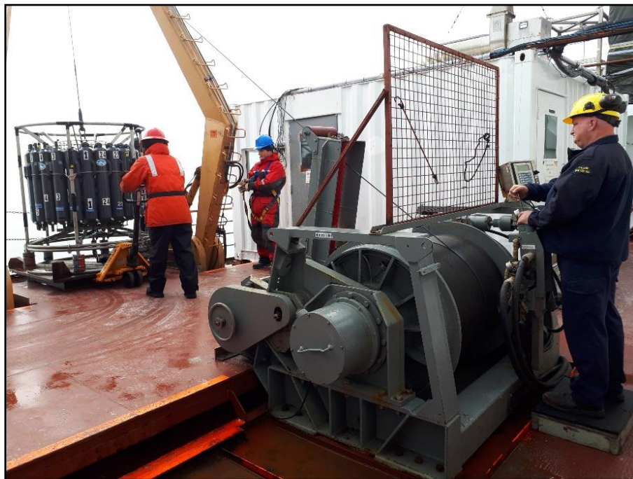
Figure 8. Rosette operation on deck with Hawboldt winch and Brooks Ocean Instrumented Sheave display box mounted on the right. (photo 2022 but similar for 2023).
