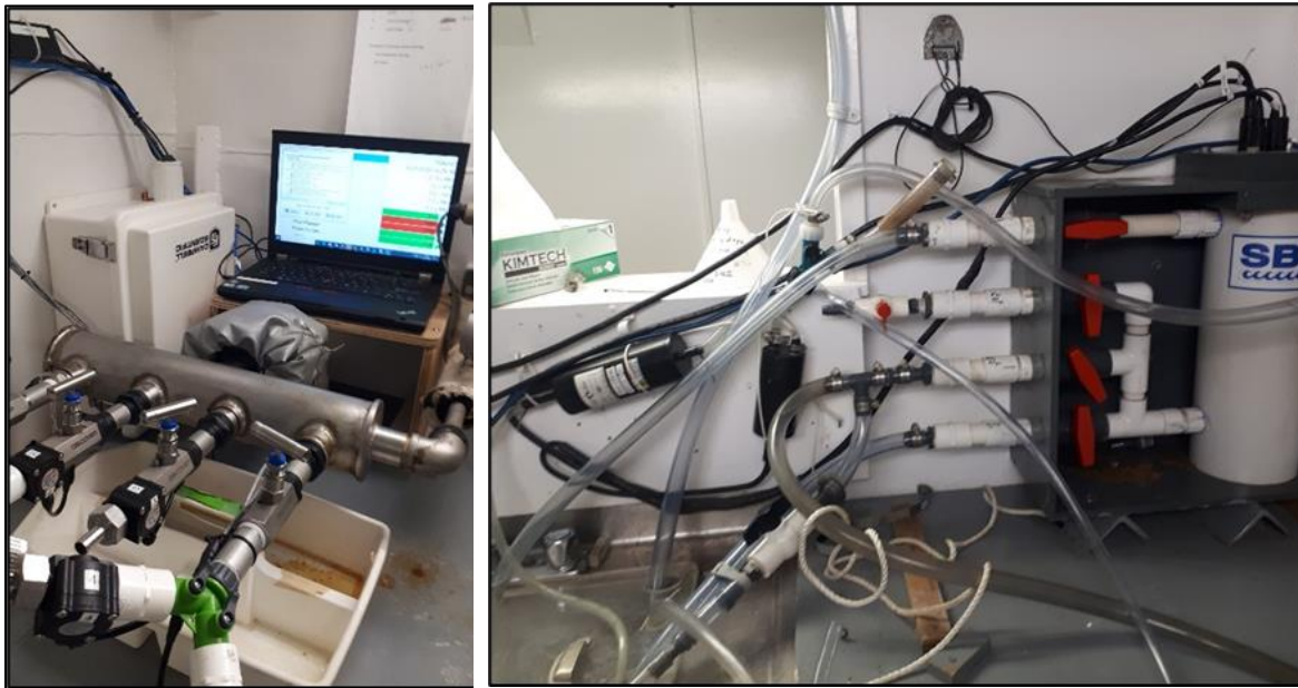
Figure A2. @Left: TSG manifold, flow meters, data logger and laptop. @Right: TSG tank and fluorometer pair with orientation to not trap bubbles and have good flow past sensor (vertical orientation for Chl-a and horizontal orientation for FDOM) (photos 2023).
