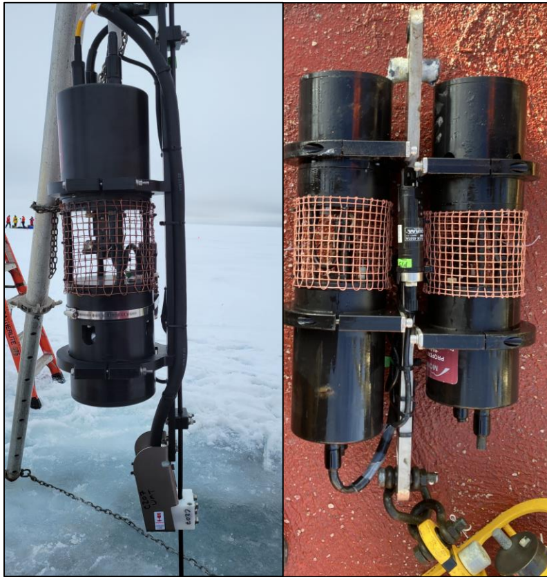
Figure 27. SAMI CO 2 being deployed on an ITP (left) and CO 2 and pH sensors after recovery on Mooring B (right).
