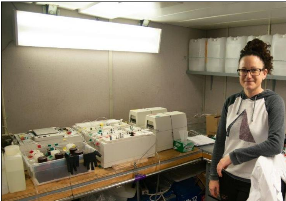
Figure 44. Nutrients analysis on the AA3. Photo by Fred Marin, 2019, but similar set up for 2023.
