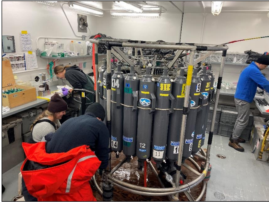
Figure 10. Water sampling around 24 bottle rosette
