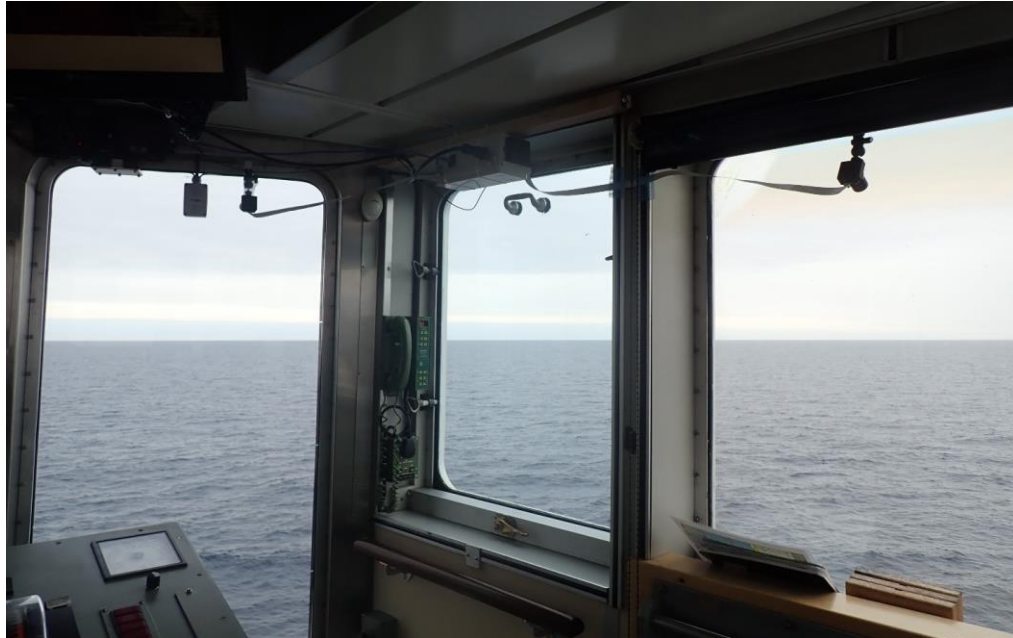
Figure 32. Location of SSICR with forward and side looking lenses on the starboard side of the bridge.
