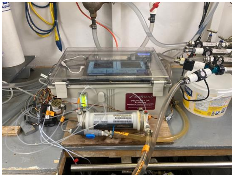
Figure 25. Shipboard underway p\text{CO}_2 environmental monitor (SUPER) system connected to the ship's seawater line (at right).
