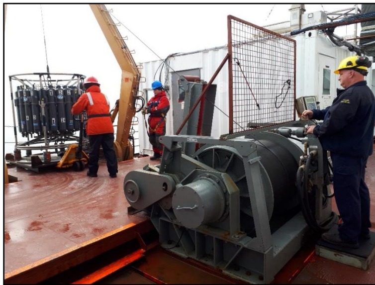
Figure 8. Rosette operation on deck with Hawboldt winch and Brooks Ocean Instrumented Sheave display box mounted on the right. (photo 2022 but similar for 2024).
