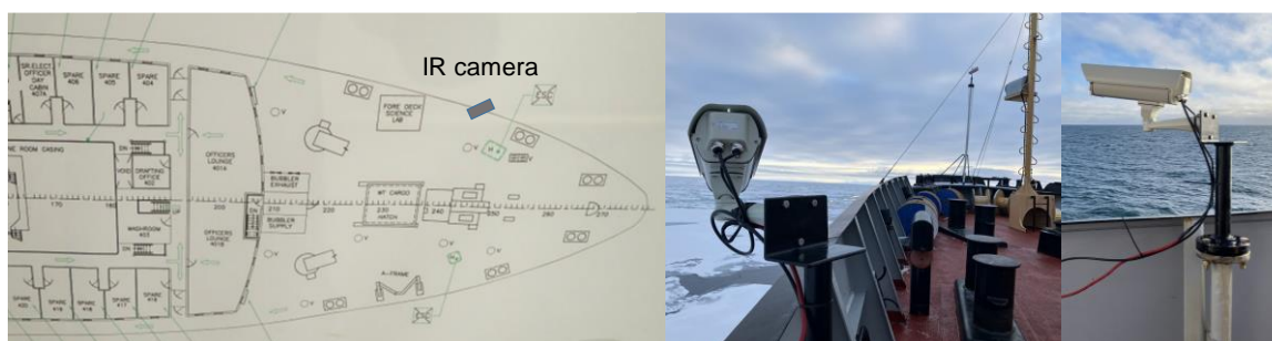
Figure 3.12.1-1. Location of the infrared camera: (left) plan view; (middle) Typical setting of the camera pointing forward; (right) camera housing attached to a fixture.
