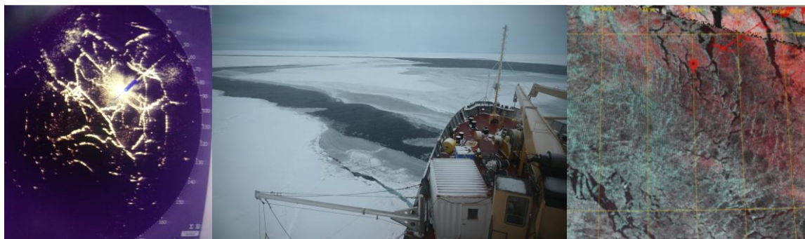
Figure 3.11.2-1. Ice-Navigator snapshot (left), photograph from the ship (center) and the SAR image (RADARSAT-2) of the same day (right)
