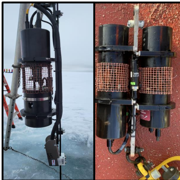
Figure 3.3.4-1. SAMI CO 2 being deployed on an ITP (left) and CO 2 and pH sensors after recovery on Mooring B (right).
