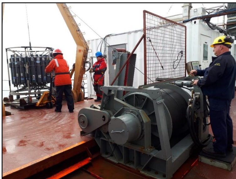
Figure 3.1-2. Rosette operation on deck with Hawboldt winch and Brooks Ocean Instrumented Sheave display box mounted on the right.
