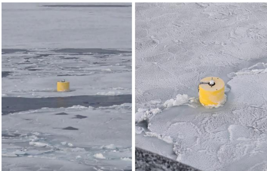
Recovery of TOP14. The TOP14 surface package recovery was a quick pick-up with no tether or profiling unit to recover. This unit also had an experimental thermistor chain on the grounding pole, which was torn off in a rafting event.
