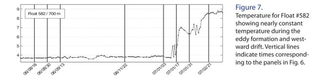
Figure 7. Temperature for Float #582 showing nearly constant temperature during the eddy formation and westward drift. Vertical lines indicate times corresponding to the panels in Fig. 6.
