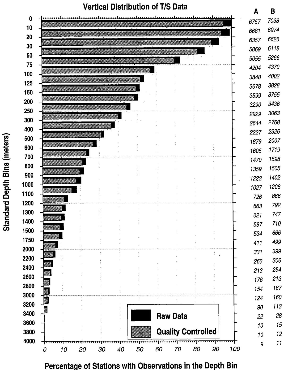
**Figure 8.** Vertical distribution of the data before QC (black), and after QC (gray). Column A shows the number of profiles with observations after QC. Column B shows the number of profiles in the original data set.
