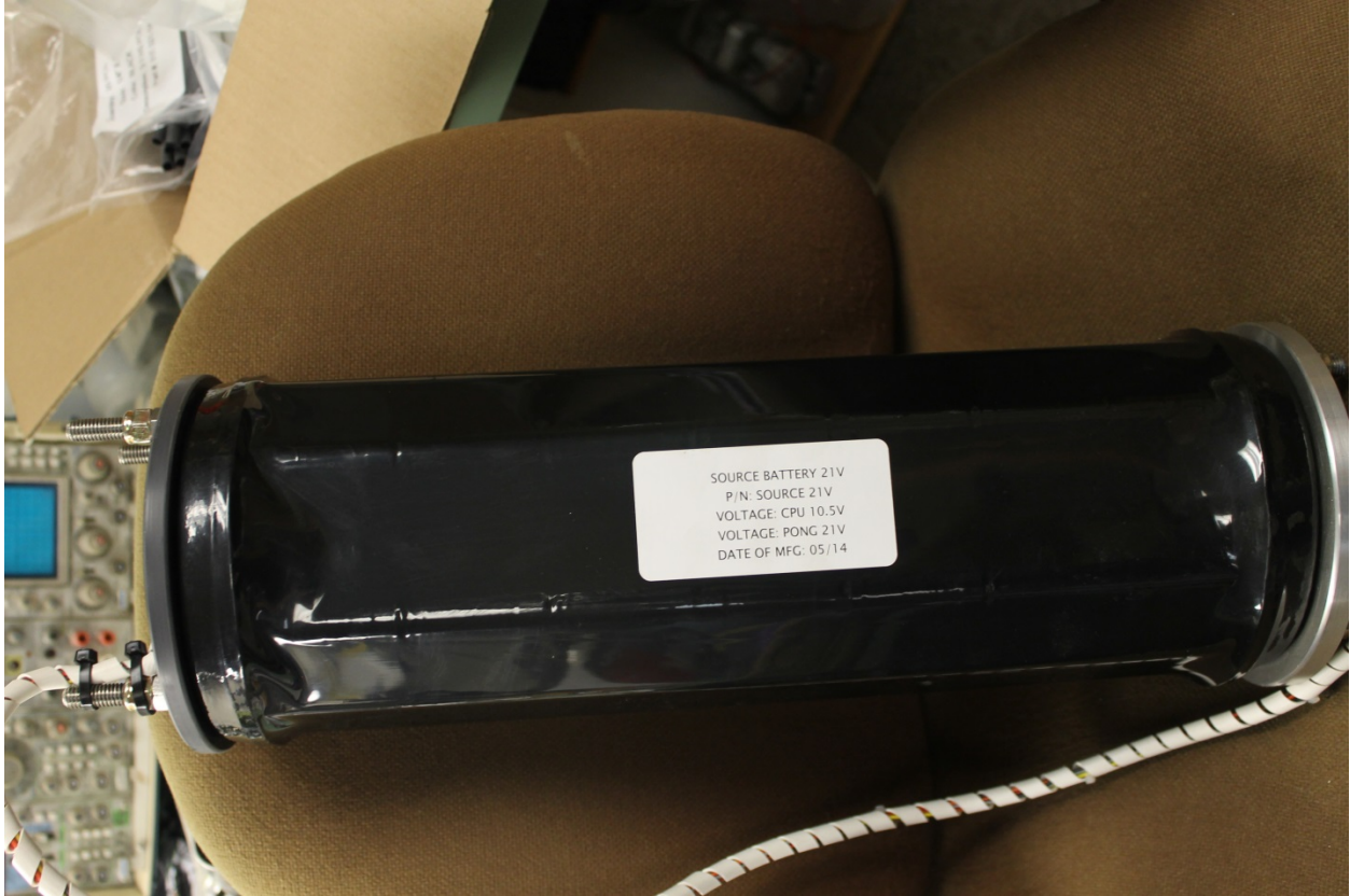
The battery is assembled and secured to the snap ring.
