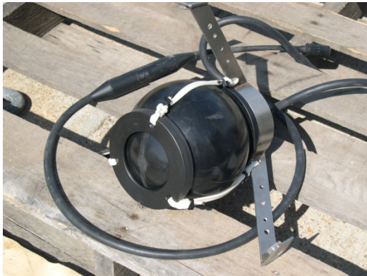
Pic. 3 Assembled Transducer, ready for mounting in the resonator.
