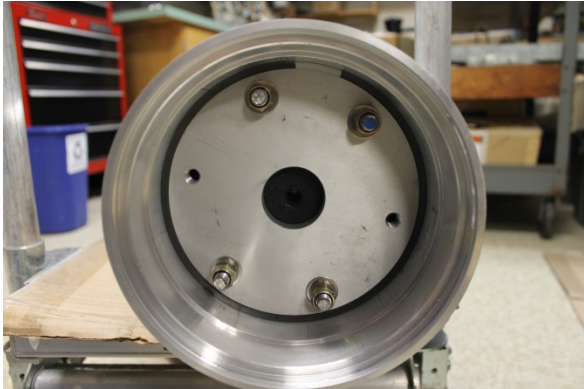
The battery is assembled and secured to the snap ring.
