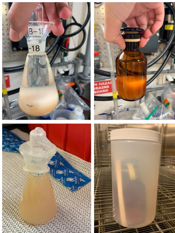
Figure 5. Oxygen sample bottle types and storage methods. (left) provided by D. Nicholson, (right) provided by D. Wellwood.
