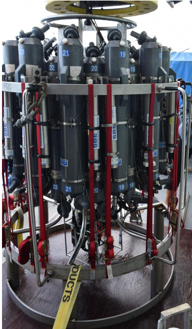
Figure 12. Microcats strapped to the rosette frame, zipties were important at top of instrument to keep tight to the frame and limit strumming.
