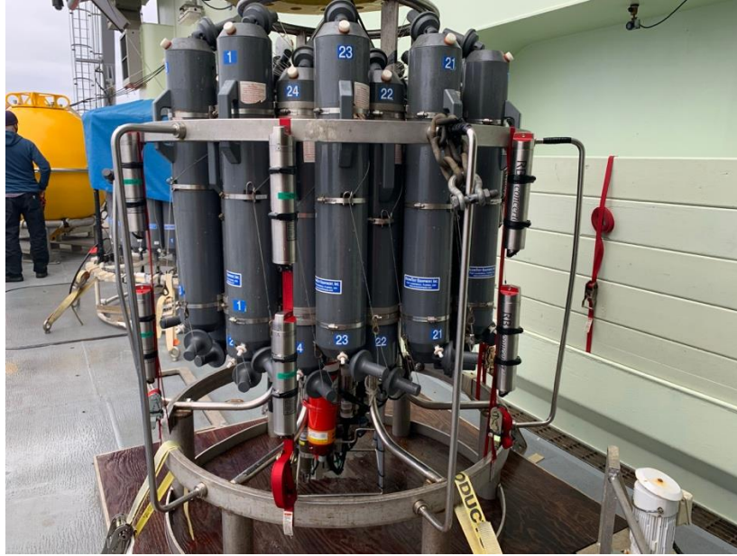
Figure 6. RBR Concertos attached to CTD rosette using ratchet straps and hose clamps. Additional steps were using 3M Super 88 electrical tape around all hose clamps to ensure screws on hose clamps stayed in place.
