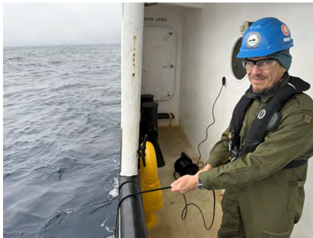
Figure 6: Over the side transducer into the port side pass through
