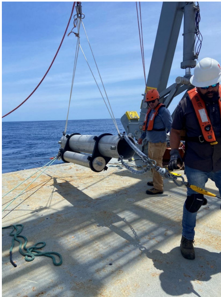
Figure 5: Photo of rigging system on source. Eduardo Jardim spliced a deployment line specific to this source. Photo by H. Furey.
