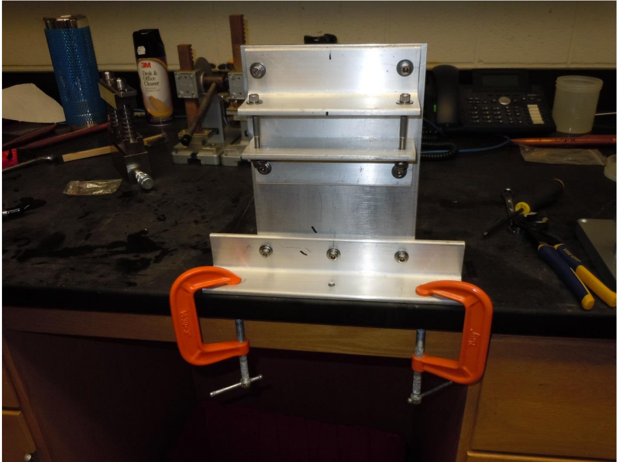
Figure 3: Aluminum Mounting Bracket for the Jaws
