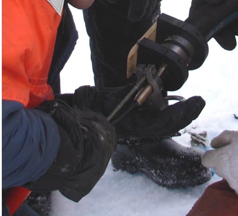
Figure 12: Attaching slip bale to cable.
