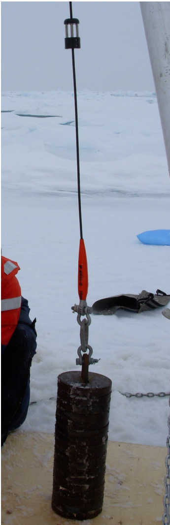
Figure 9: Anchor connection on wire and correct bumper placement.
