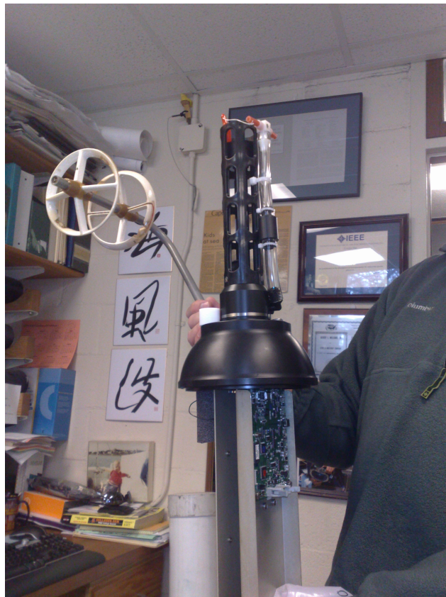
Fig. 5. MAVS, CTD, and top endcap of Ice Tethered Profiler. MAVS velocity sensor is the white rings. A 3-axis rate gyro is mounted to the chassis.
