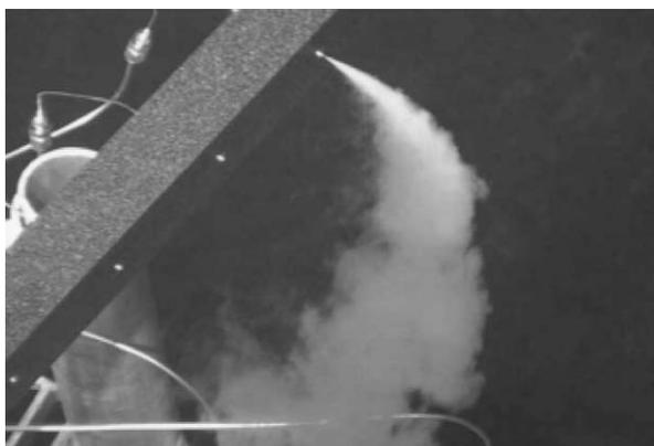
Fig. 2. A jet of SF<sub>6</sub> tracer issuing from a 50-μm orifice.
