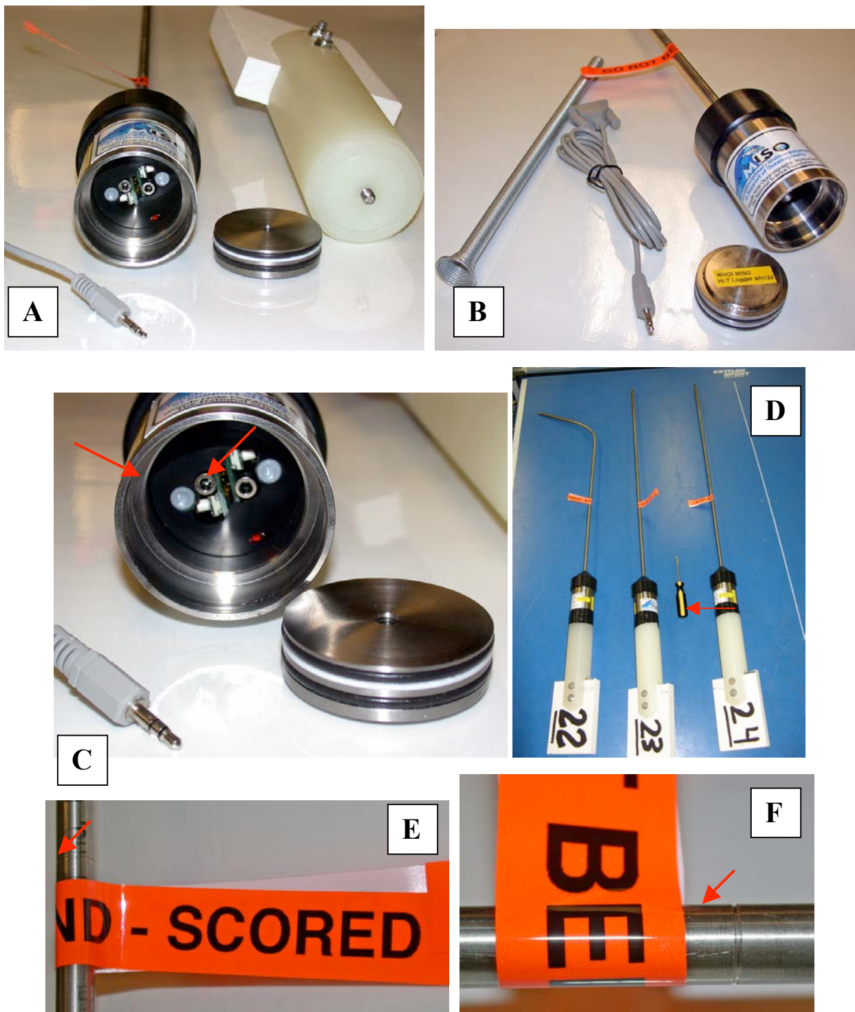
Figure 4. (A) Old-style housing, syntactic foam handle, and endcap. Download cable - mini-RCA plug - shown that connects to Onset™ logger chips in the housing. (B) Logger components: housing, end-cap, serial download cable, tubing bender. Each housing is serialized as is the end-cap. (C) Close up of housing insides, red arrow points to the connectors on each Onset™ recording chip. (D) Loggers ready for deployment, note 'J' bend in left-most logger. Red arrow points to electrical tape used to ensure that housing and handle do not unscrew. (E&F) Close-ups of scoring on the tubing (red arrows).
