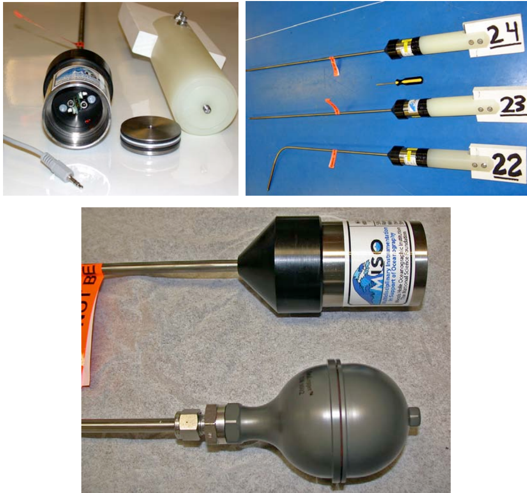
Figure 2. (top) Cylindrical (old-style) high-T fluid temperature loggers currently manufactured and serviced by the MISO Facility. These loggers have been modified to accommodate two (2)- 32k Onset™ logging chips. When/if the tips are broken on recovery they must be returned to the facility for machining, re-welding and re-certification and installation of new logging chips. (bottom) Old style (cylindrical with MISO label) and new-style (spherical, gray housing) logger housings.
