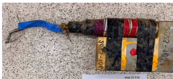
Logger recovered with tip broken off
