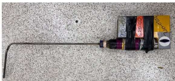
Logger recovered with tip largely intact
