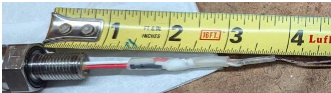
Figure 20. Relocated Cold Junction Thermistor
