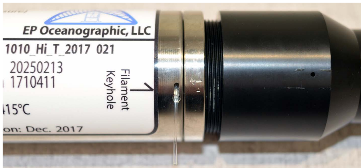
Figure 1. Housing showing etched arrow marking alignment of locking filament entry hole so that it can be aligned properly with the filament keyhole
