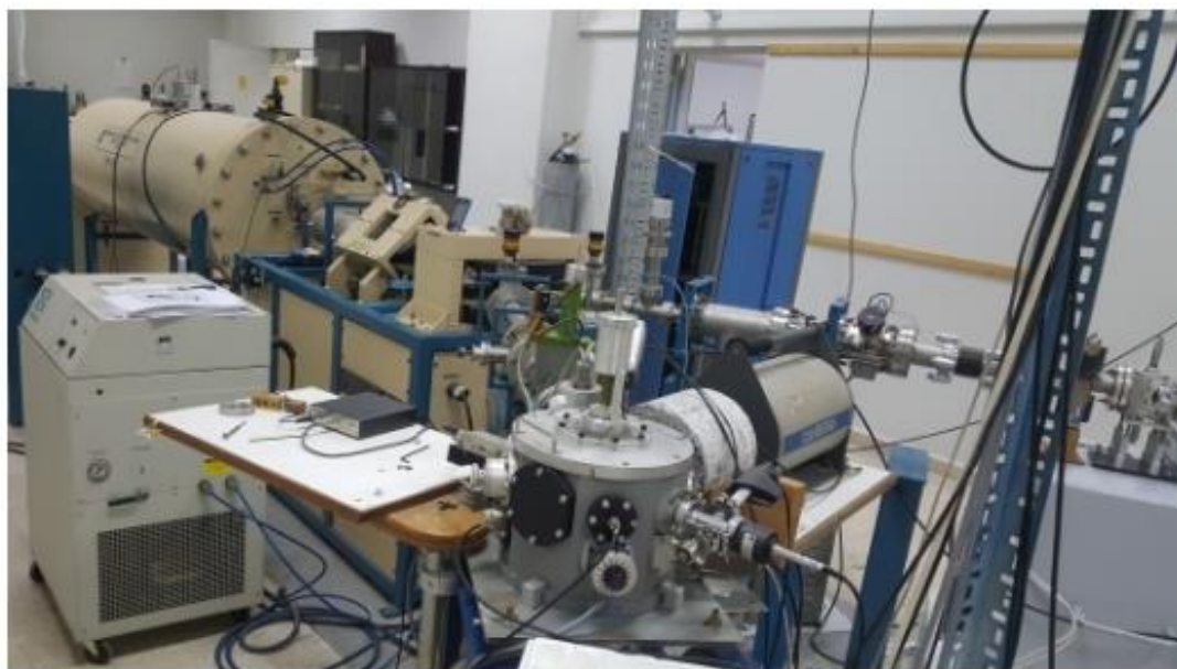
The structure of an ion beam accelerator at a laboratory belonging to the Lebanese Atomic Energy Commission. (Photo: Lebanese Atomic Energy Commission)
