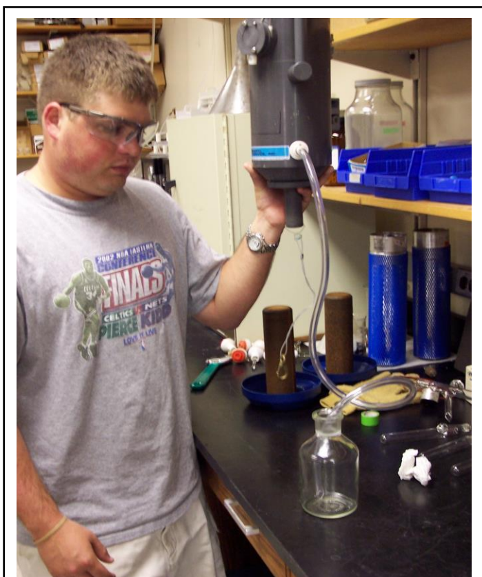
Figure 1. Filling bottle from Niskin. Note the tygon tube is at the base of the bottle. Count how long it takes for the bottle to fill, and then allow the water to overflow the bottle for half this time. Pull out the tygon tube, and remove enough water to leave an approximately 3/8" headspace below the stopper joint.
