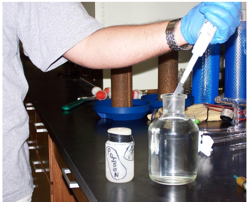
Figure 3. Addition of \text{HgCl}_2 to sample bottle after headspace has been created.
