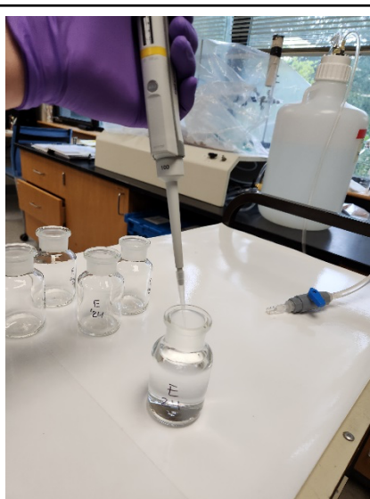
Figure 4. Addition of \text{HgCl}_2 to sample bottle after headspace has been created.
