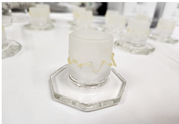
Figure 2. Properly greased stopper
