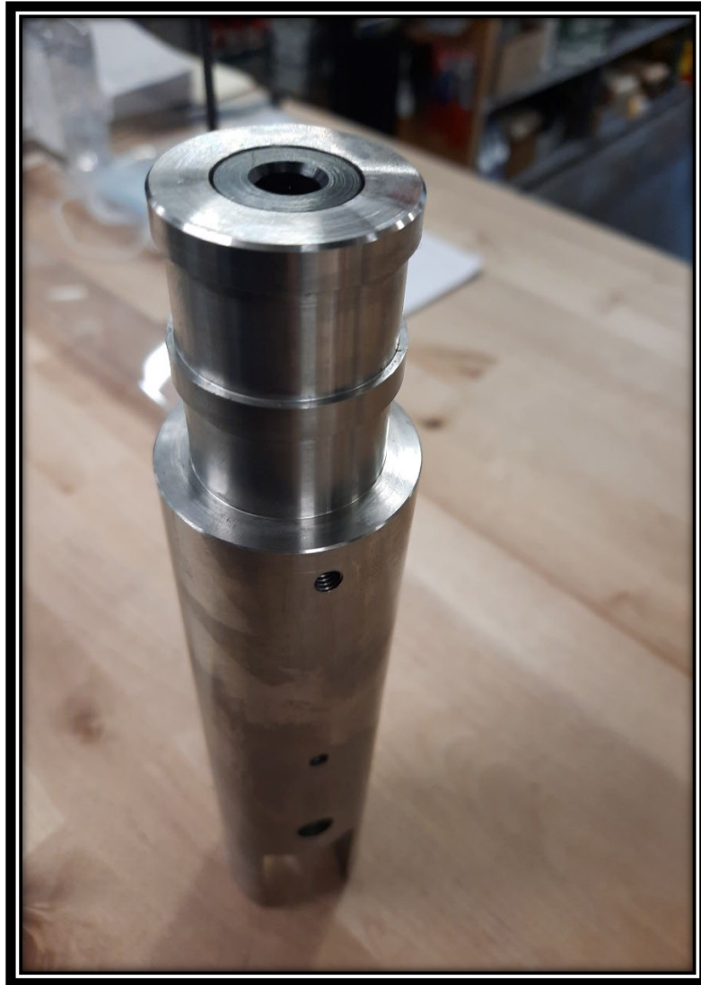
CTD termination with adapter plug
