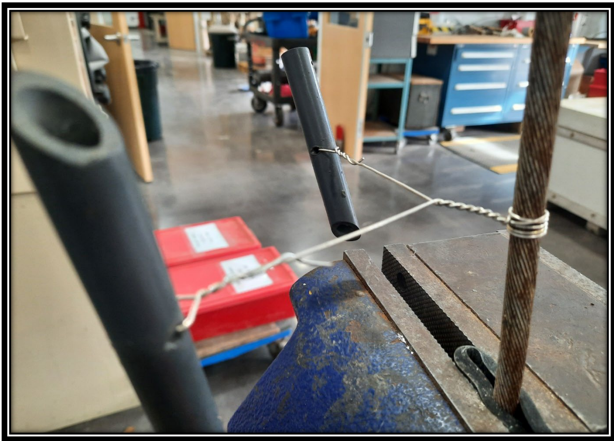
.322 cable seized with buss wire
