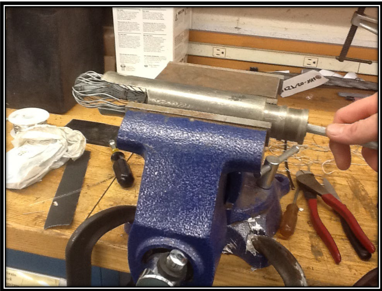
Birdcage being pulled into termination body
