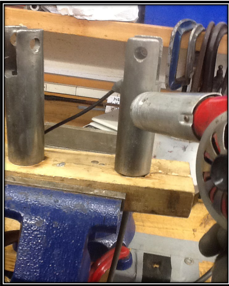
Heating the termination body will allow Cerrobend it to cool evenly
