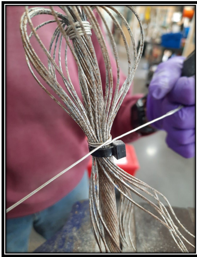
Outer layer of armor wires folded over seizing to form first birdcage
