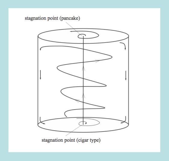
The swirling, overturning circulation observed in ocean eddies can be modeled in a rotating cylinder driven by a stress at the top surface. (Pratt and Rypina)
