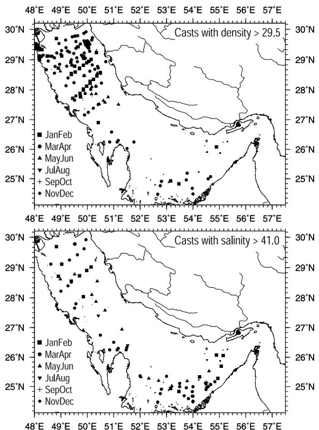
**Figure 6.** Most stations with at least one sample having density  $>29.5$  occur in the northern end of the Gulf, and most were collected in the January–April period. High salinity stations ( $S > 41$  psu) are equally distributed between the northern Gulf and the banks along the south coast. Almost no stations in the axial trough or the western approach to the Strait have high density or salinity.
