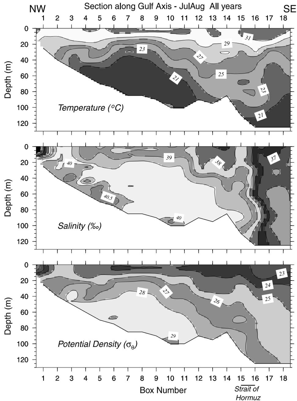
**Figure 7d.** Axial section in July–August shows that the southeast end of the front separating modified IOSW from Gulf Deep Water has moved up the basin to at least box 12. Warm, low-salinity surface water has been stirred downward in the region to the west of the Strait (boxes 12–15). Solar heating has warmed the complete water column lowering overall density compared to previous months.
