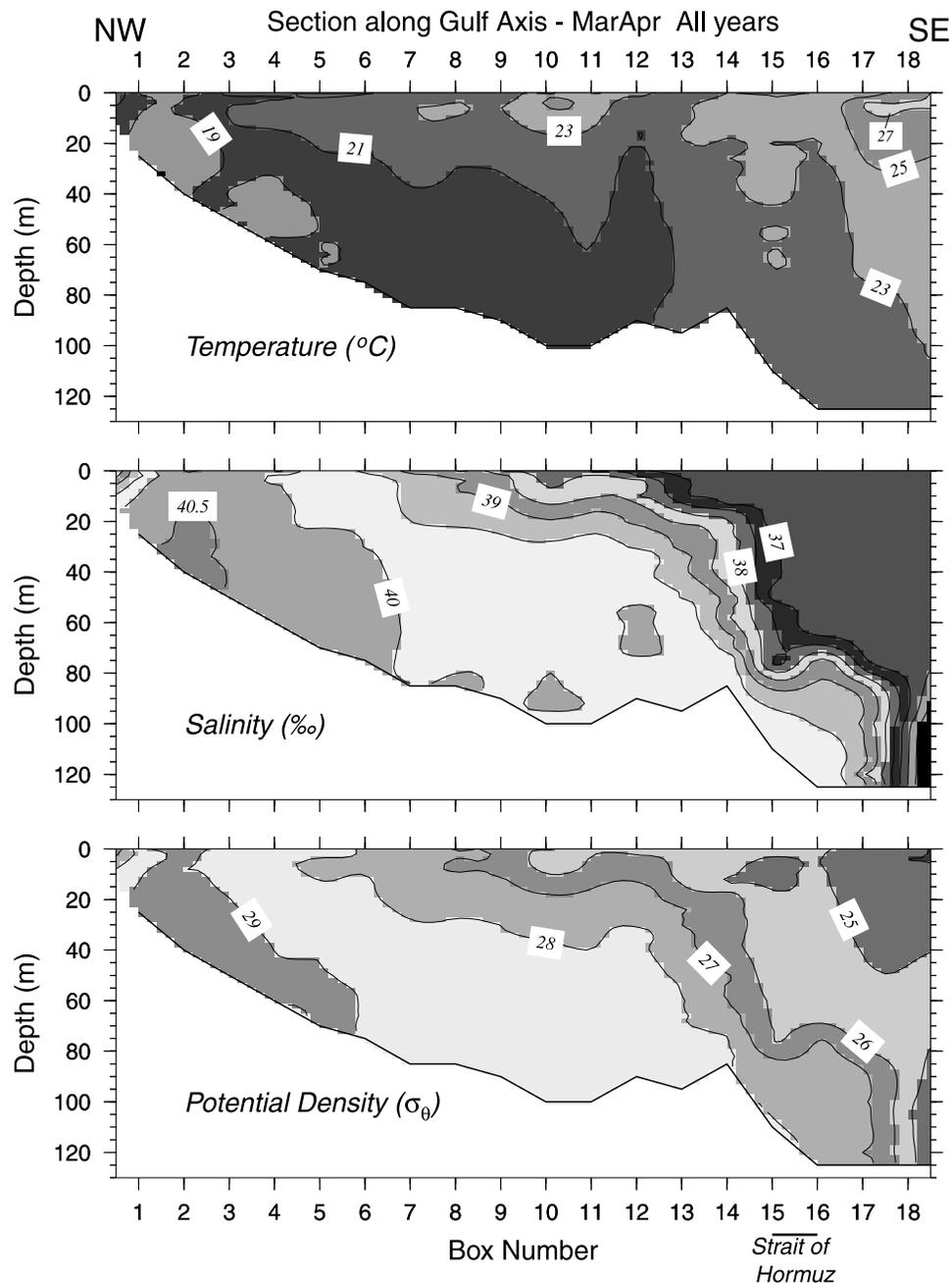
**Figure 7b.** Axial section for March–April shows cold, saline water still outcrops at the sea surface of the Tigris-Euphrates-Karun delta. Warm, low salinity IOSW at the sea surface has moved farther up the Gulf.
