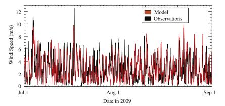
**Fig. 2.** Observed (black curve) and predicted (red curve) wind speed at N1734 versus time. The squared correlation between the model and data  $r^2$ =0.26, the ratio of the predicted to observed standard deviation  $\sigma_{ratio}$ =1.0, the bias=0.0 m s<sup>-1</sup>, and root-mean-square model error rmse=1.9 m s<sup>-1</sup>.
