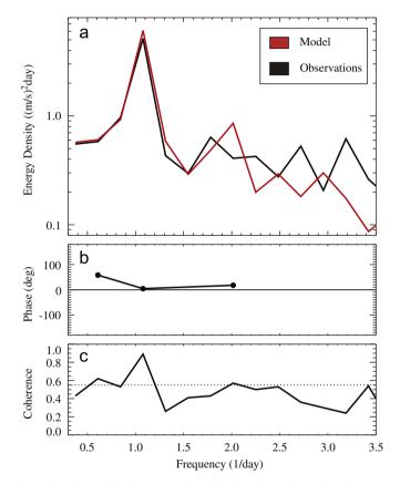
**Fig. 3.** (a) Observed (black curve) and predicted (red curve) wind-speed energy density at N1734 (20 degrees of freedom), (b) phase between observations and predictions (positive values suggest the observations lead the predictions), and (c) coherence between observations and predictions versus frequency. Phases are shown only when the coherence is significant (95% significance level shown by the horizontal dotted line in (c)).
