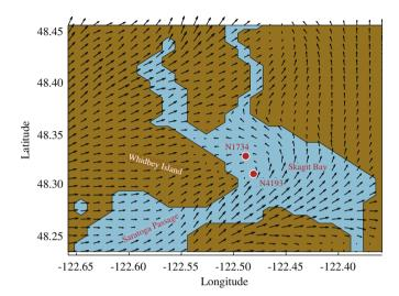
**Fig. 8.** Modeled 1-h-averaged wind speeds and directions (length and orientation of vectors) for a case with large-scale winds from the west-southwest. Brown is land and blue is water. Locations of N1734 and N4193 are shown by the red circles. Maximum wind speeds for this case are about 8 m s<sup>-1</sup>. Winds from the WSW and SW funnel through Saratoga Passage, creating a separation zone behind Whidbey Island.
