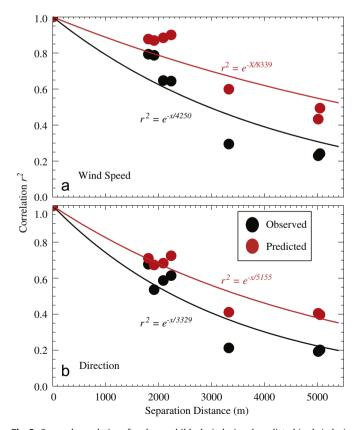
**Fig. 5.** Squared correlations for observed (black circles) and predicted (red circles) (a) wind speed and (b) wind direction at all pairs of anemometers on the tidal flats during July 2009 versus separation distance between each pair of locations. The best-fit exponential decays are shown by the black (observed) and red (predicted) curves.
