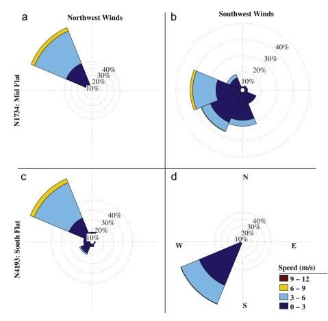
Fig. 7. Wind roses for modeled winds at (a and b) N1734 and (c and d) N4193 when (a and c) winds at N1734 are from the northwest and when (b and d) the winds at N4193 are from the southwest.
