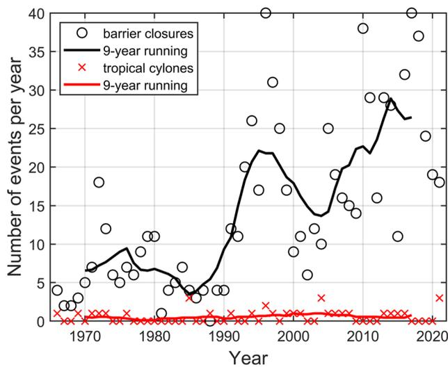
**Figure 3.** Annual frequency of New Bedford Hurricane Barrier closures (USACE, 2022b) and tropical cyclones (TCs) passing within 200 km from 1966 to 2021 (Landsea & Franklin, 2013), along with 9-year running averages.
