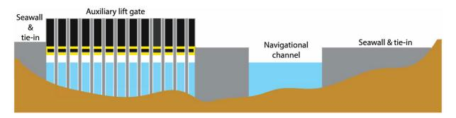
**Figure 1.** Schematic cross-section of a storm surge barrier system for an estuary with a wide ocean entrance. It includes auxiliary gates intended to reduce flow obstruction during non-storm periods and a wide navigation channel (which also has large gates, not pictured). A similar barrier is proposed for Jamaica Bay, New York City (USACE, 2022a).
