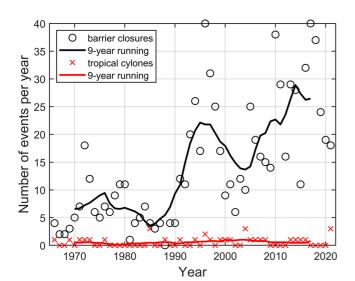
**Figure 3.** Annual frequency of New Bedford Hurricane Barrier closures (USACE, 2022b) and tropical cyclones (TCs) passing within 200 km from 1966 to 2021 (Landsea & Franklin, 2013), along with 9-year running averages.
