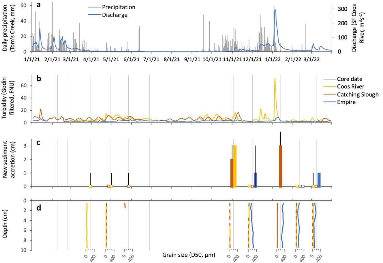
**Fig. 4** Timeseries of hydrological and sediment observations in Coos Bay, including daily precipitation at the Tom's Creek meteorological station and South Fork Coos River discharge (a; duplicated from Fig. 3 for comparison), turbidity (b), new sediment accretion (c), and median grain size profiles (d). In panels b–d, core collection dates are indicated by vertical grey lines. In panel c, open squares represent
