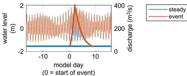
**Fig. 2** Timeseries of modeled water level (thick lines) and Coos River discharge (thin lines) during typical winter conditions (“steady,” blue) and high river discharge conditions (“event,” orange) at the Coos River study site
