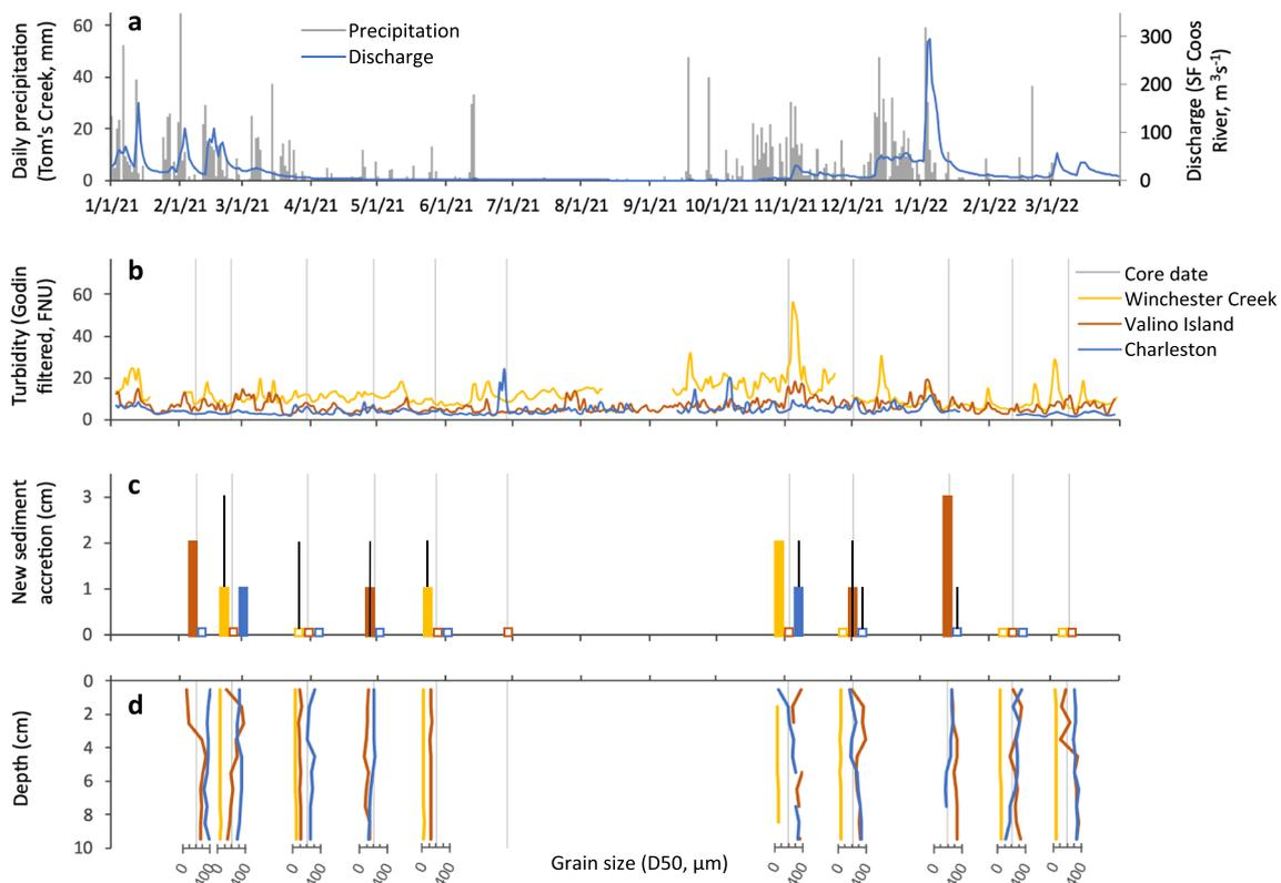
**Fig. 3** Timeseries of hydrological and sediment observations in South Slough, including daily precipitation at the Tom's Creek meteorological station and South Fork Coos River discharge (**a**), turbidity (**b**), new sediment accretion (**c**), and median grain size profiles (**d**). In panels **b–d**, core collection dates are indicated by vertical grey lines. In panel **c**, open squares represent cores showing no new sedi-
