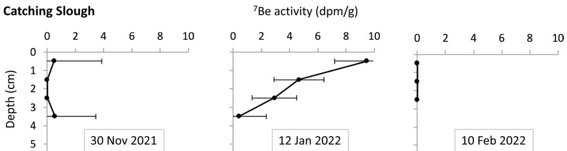
**Fig. 5** Example <sup>7</sup>Be profiles at Catching Slough. In late November 2021 (left), the near-zero activity of <sup>7</sup>Be indicates no recent sediment deposition. In mid-January 2022 (middle), elevated <sup>7</sup>Be activity shows the deposition of 3 cm of new sediment. The following month
