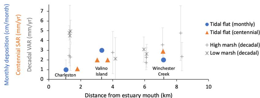
**Fig. 8** Comparison of along-estuary patterns of sedimentation in South Slough over monthly and centennial timescales. Blue circles ( $n=3$ ) show maximum monthly deposition observed at the South Slough tidal flat coring sites during the study period. Mean centennial sediment accumulation rates (SAR) from Eidam et al. (2024) are
