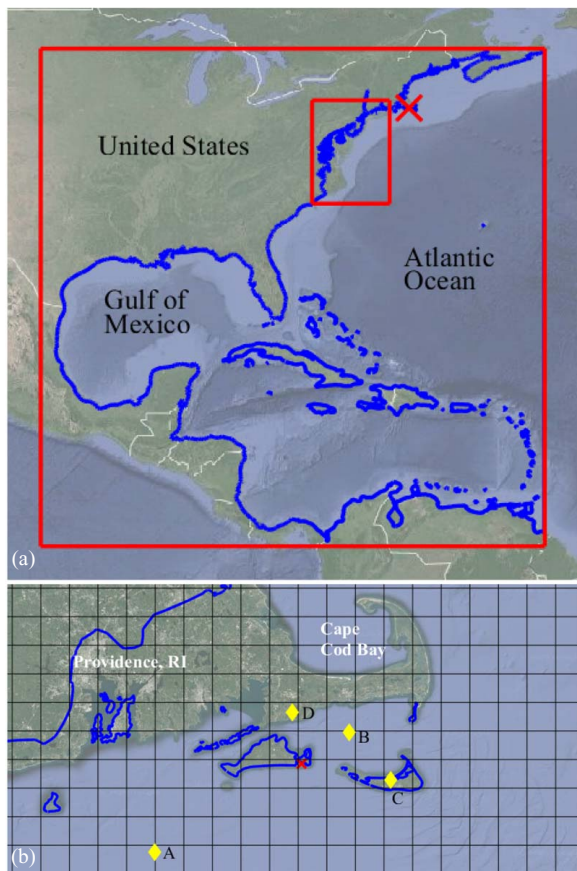
Fig. 3. (a) Map showing the outline of the ADCIRC model domain boundaries in dark blue and the boundaries of the two wind and pressure field domains in red. A red X demarks the study area. (b) Map showing a more detailed view of the project area, with the ADCIRC model domain boundaries in dark blue and the black gridded lines showing the grid cells for the Level 1 wind and pressure fields. Winds were observed at the four locations marked with yellow diamonds, with waves observed at yellow diamonds A and B. The red X demarks the study area.
