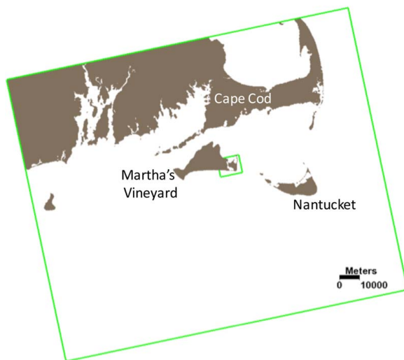
Fig. 7. Southern Massachusetts grid (SMA) (outer green box) and the higher-spatial resolution Katama Bay grid (KB) (inner green box) used for STWAVE.
