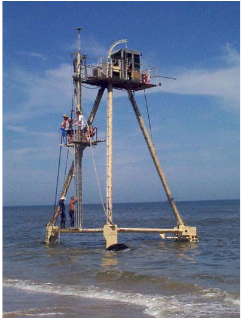
Fig. III.D.12. The US Army Corps of Engineers Field Research (USACE) Facility's Coastal Research Amphibious Buggy (CRAB). This deployment and retrieval platform is a tower on three wheels, hydraulically driven by a diesel engine located on the operations platform 11 m above the seabed. The CRAB can operate in 2 m high breaking waves in 10 m depth of water, with GPS-positioning accuracy to deploy fluid- and sediment-boundary layer sensors. The CRAB has also been used to measure monthly bathymetric changes at the Duck, NC site over the past 25 years.
