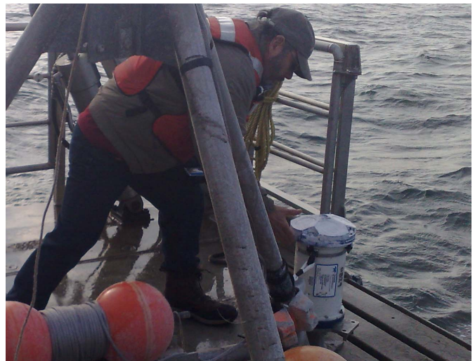
Fig. 2. The ADCP transducers are covered with Desitin™ to inhibit barnacle settlement.
