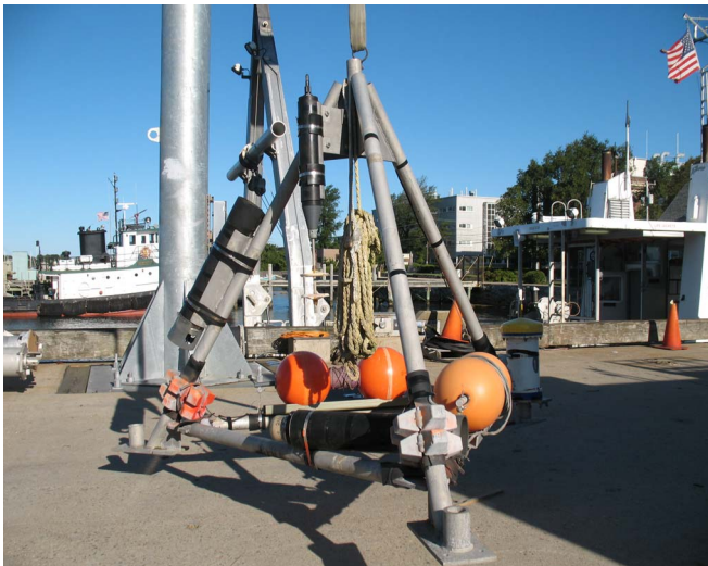
Fig. 1. The small tripod supports a MAVS and an ADCP sensor for current, wave, and turbulence measurements. The ADCP is on the far footpad, the MAVS is mounted to the vertex, and two acoustic command releases, one horizontal on the near strut and the other vertical on the left diagonal can activate the pop-up floats each with a pair of orange balls and a lift line wrapped around its axle.
