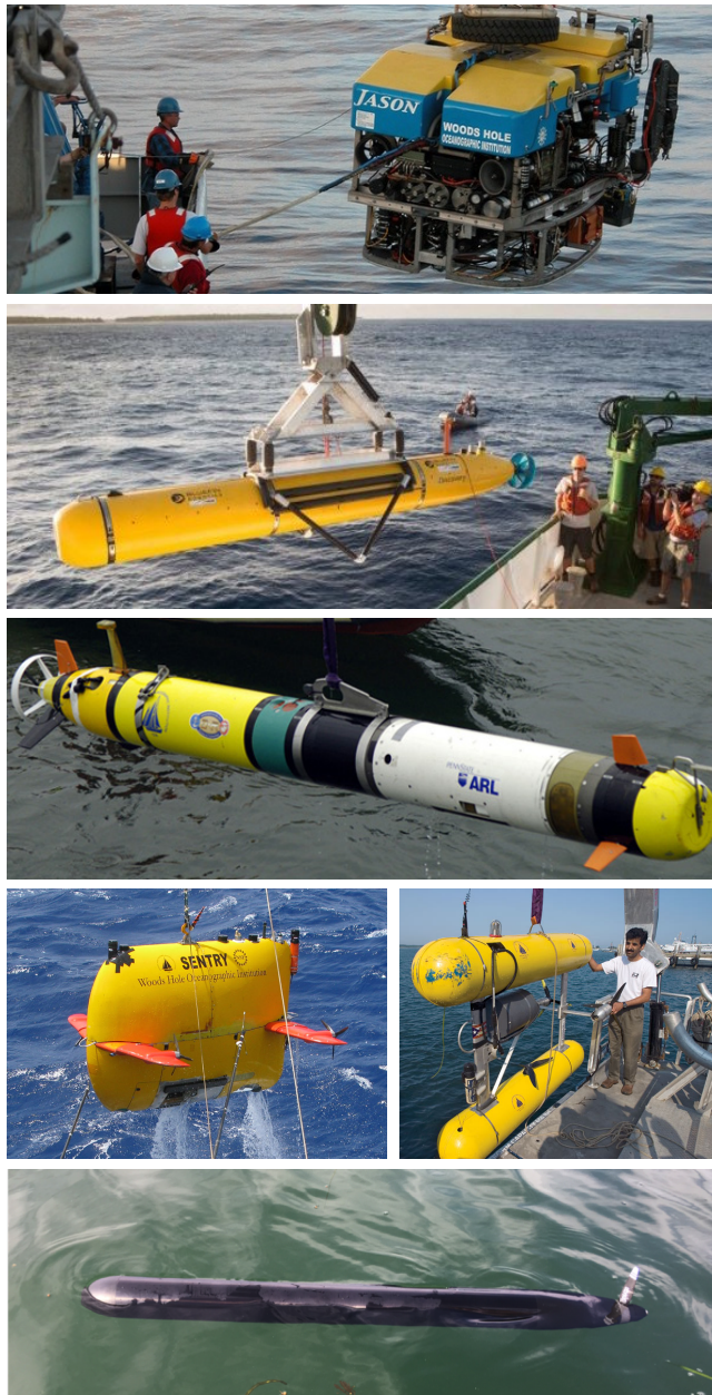
Fig. 1. A variety of unmanned underwater robots with a variety of propulsion systems for performing a variety of tasks. From top to bottom: ROVs like JASON are controlled by an operator over a tether and use a variety of thrusters to hold station over areas of interest. AUVs are designed for long transits and large area searches are streamlined and can employ a vectored thruster like a Bluefin or a propeller with aft fins, and sometimes even forward fins, like a REMUS. AUVs designed as slow-moving and highly stable imaging platforms, like Sentry and SeaBed, use multiple thrusters to maintain low-speed maneuverability and have large separation between their centers of mass and buoyancy. The APS vehicle is designed to be both streamline and to maintain maneuverability at low speeds while only requiring a single degree of freedom asymmetric propeller to maneuver.
