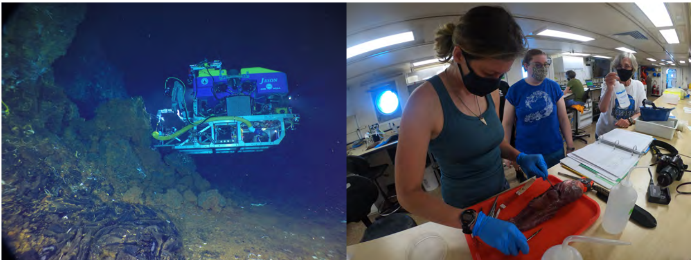
Left: ROV Jason collecting samples at the 9°50'N EPR vent field. A new high-capacity suction sampler (yellow tube running aft to fore), designed by Mario Fernandez, was used to capture large fish for the vent parasite project. Photo courtesy of NDSF ©Woods Hole Oceanographic Institution. Right: MIT-WHOI Graduate Student Lauren Dykman in the main lab of R/V Roger Revelle dissecting a vent fish that was collected by the new suction sampler. Photo: Zoe Yin.
