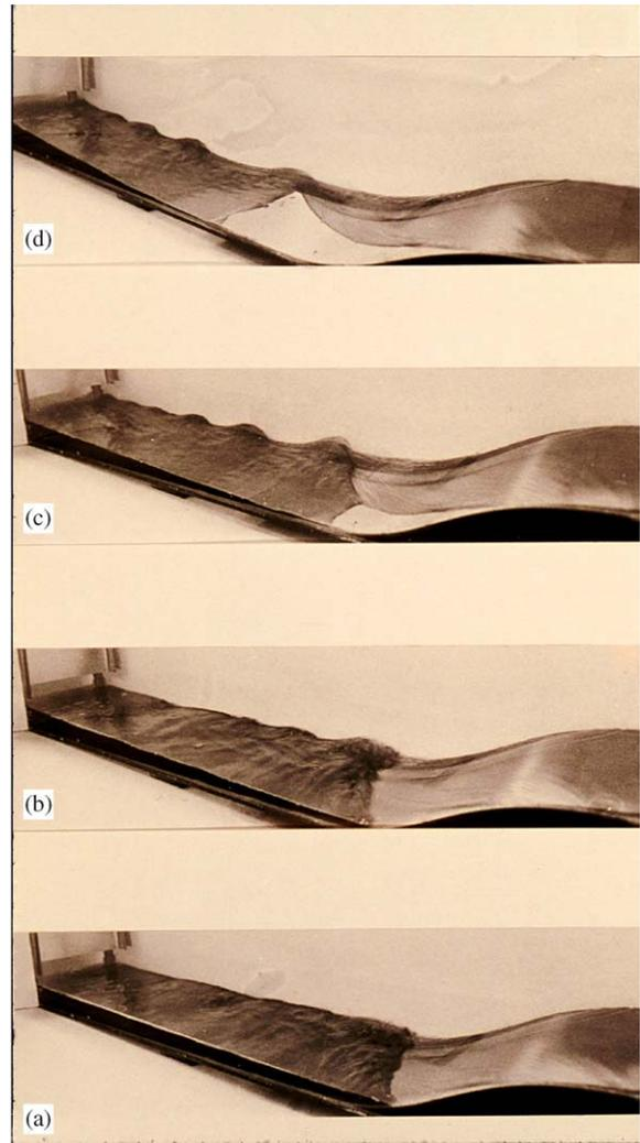
Fig. 4. Photo of rotating hydraulic jump in laboratory channel (Pratt, 1987). Fluid flows from right to left, spilling down an obstacle. At the base of the obstacle is a hydraulic jump, shown at increasing rotating rates from (a) to (d). In (c) and (d), where the spilling flow separates from the near wall, the jump is transverse.
