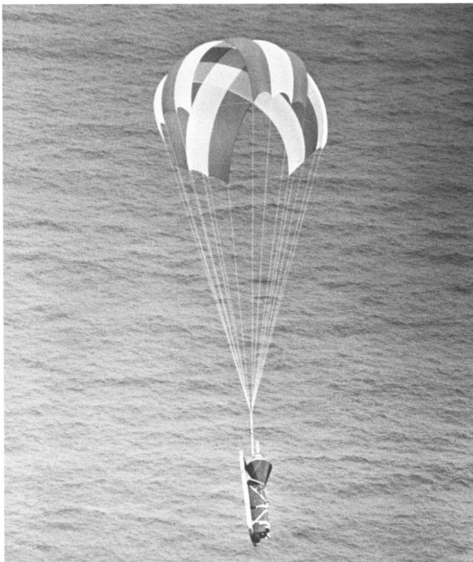
Fig. 2c. A static line connected to the ramp causes the parachute to deploy seconds after launch.
