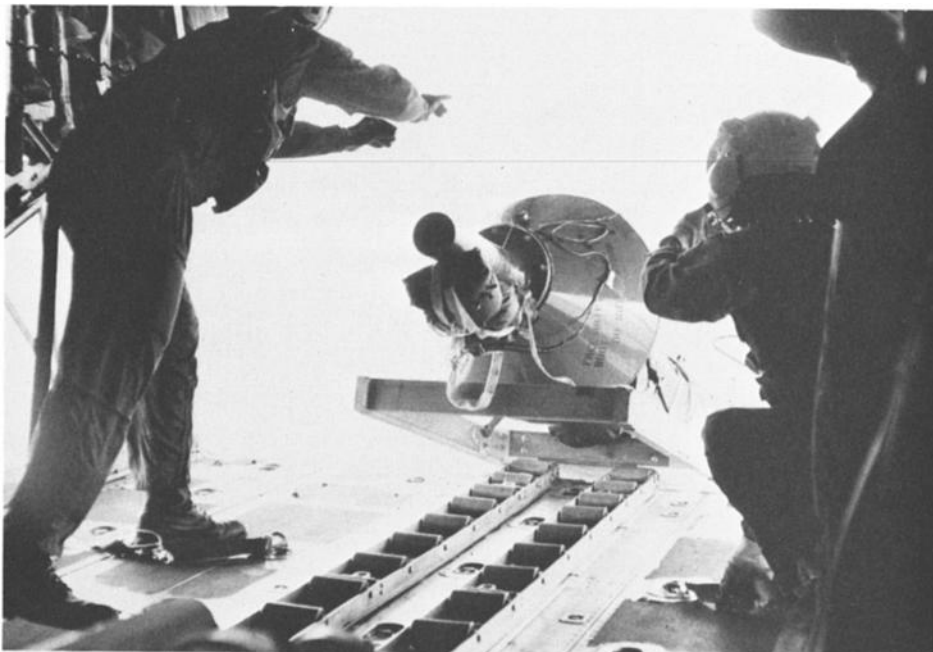
Fig. 2b. Launch procedure consists of lowering the ramp into a horizontal position and pushing the buoy out the back of the aircraft.
