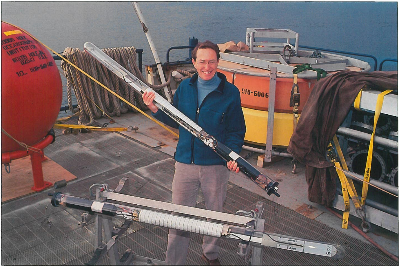
Phil Richardson hefts a RAFOS float aboard R/V Knorr.
