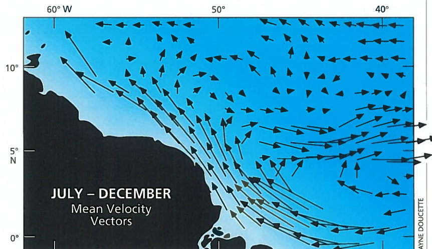
Mean velocity vectors calculated by grouping all available surface-drifter velocity measurements from 1983 to 1993 into 1°-by-1° bins. The newer data, which are similar to historical ship drifts, include trajectories in several retroflexion eddies and show that on average the North Brazil Current runs continuously up the coast into the Guyana Current, with some flow peeling off and feeding into the countercurrent. The mean northwestward current is partly an artifact of averaging the clockwise rotating swirl velocity of several eddies as they drifted northwestward along the coast.
